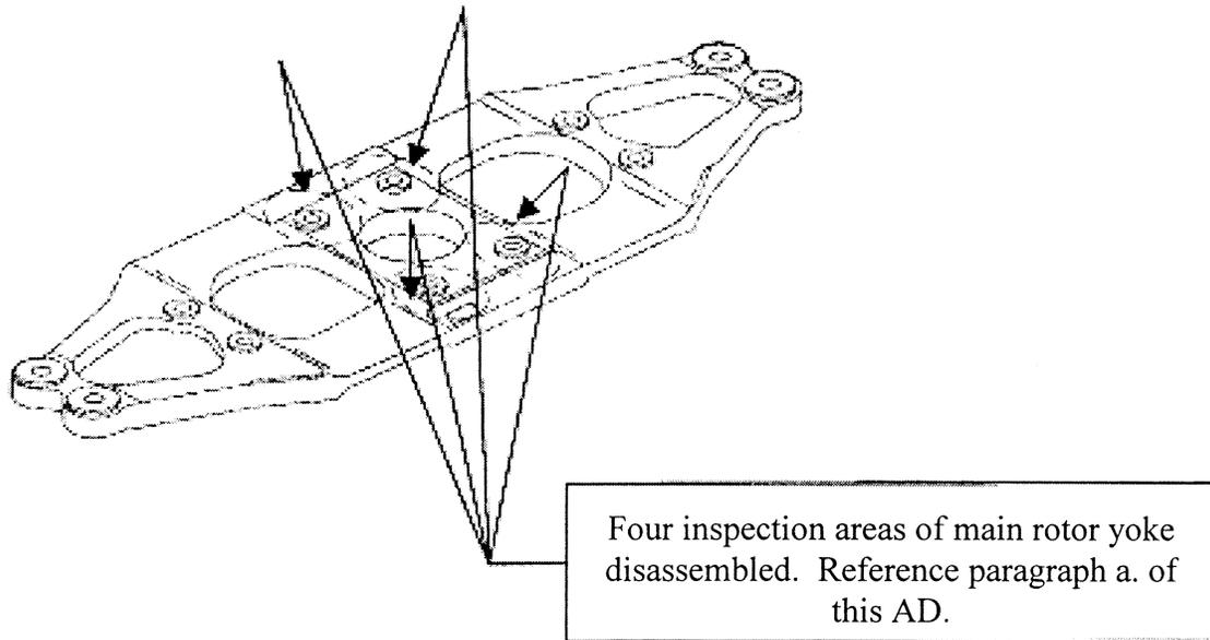
**Figure 3. Main Rotor Yoke Inspection Areas**
